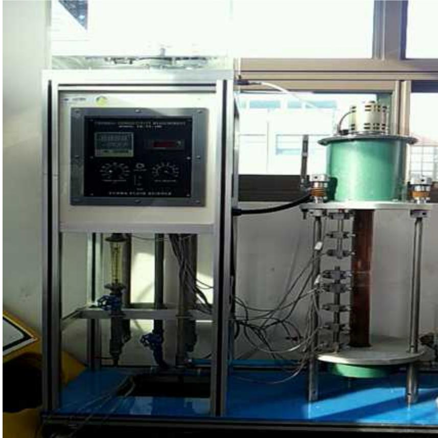
Fig. 9-3. Thermal Conductivity Measuring Apparatus.
