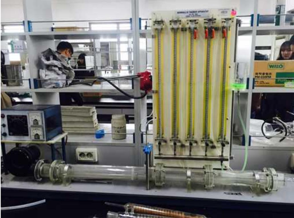
Fig. 5-1. Bernoulli Theorem Apparatus
