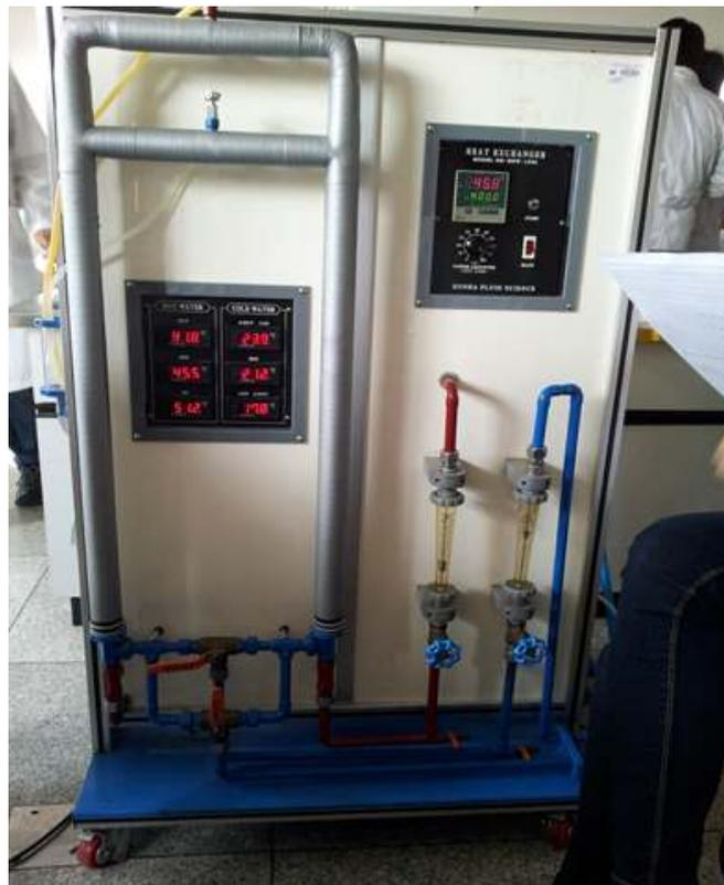
Fig. 8-1. Double Pipe Heat Exchanger
