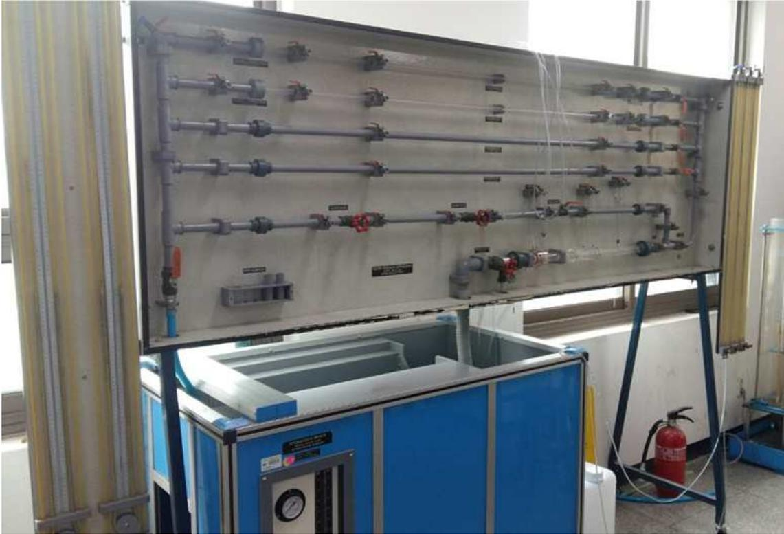
Fig. 4-1. Losses in Pipe Bend Apparatus.
